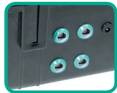
Up to 4 sensor inputs, including voltage supply for all sensors
