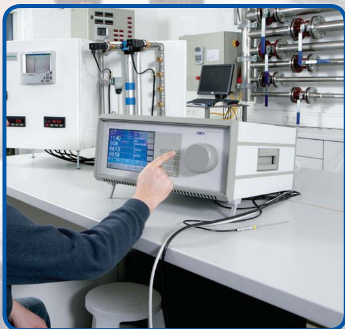
Calibration range: from -80 to 20 °Ctd Accuracy of the DKD reference: 0.1 °Ctd
