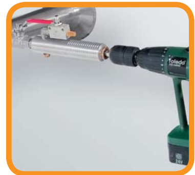
Drilling under pressure
